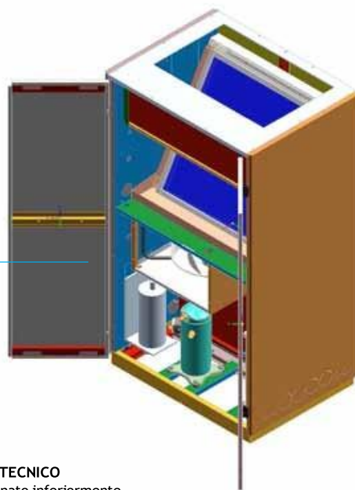
TECHNICAL COMPARTMENT Positioned in the lower section for easiest maintenance
